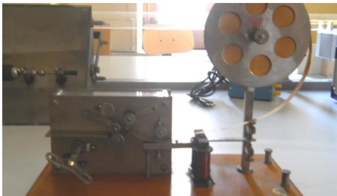
**Fig 7 Morse telegraph, tool used by E. Boggio Lera in his wireless telegraphy experiments and made working by a group of students of the school, to redo the same experiments on 8 and 9 June 2012.**
