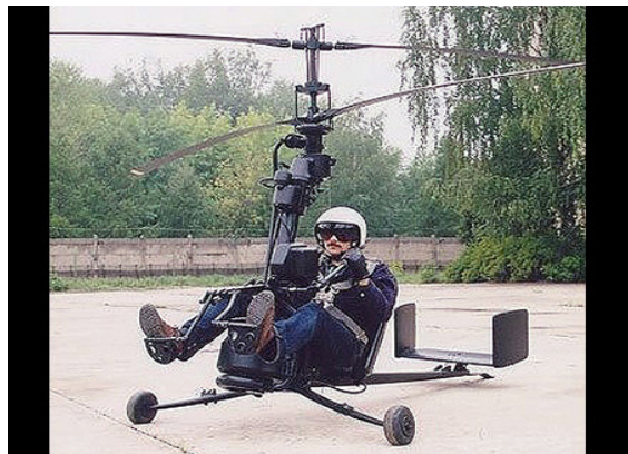
Fig. 6. KA-56- A modern "portable" (it weighs 485 pounds) helicopter
