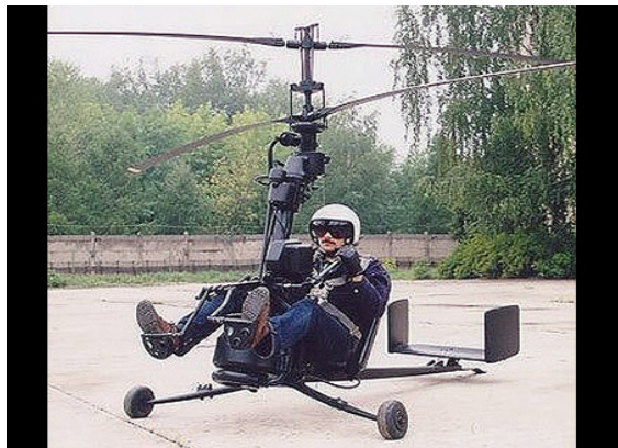
Fig. 6. KA-56- A modern "portable" (it weighs 485 pounds)
