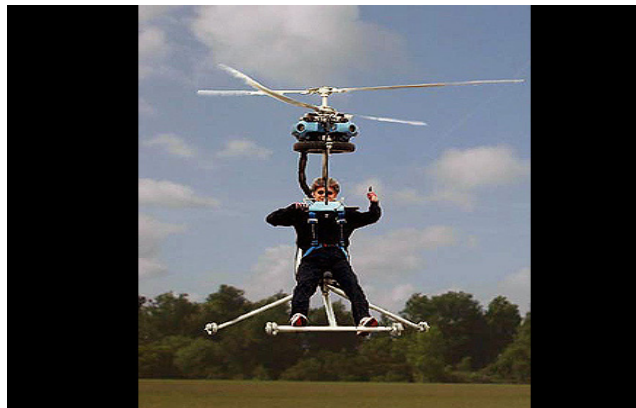
Fig. 7. GEN H-4 world's smallest co-axial helicopter (still weighs 155 pounds).
